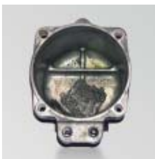
Abrasion with compressor damage
