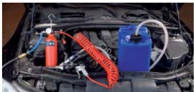
Flushing with flushing solution
