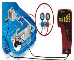
A must have tool for the A/C technician
