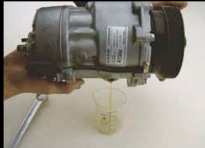
3. Drain compressor completely
