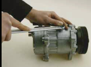
1. Loosen drain plug
