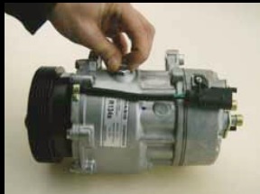
6. Put drain plug back into compressor
