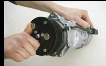
8. Turn the compressor 10 times to distribute the oil
