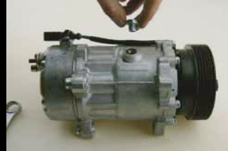
2. Remove drain plug
