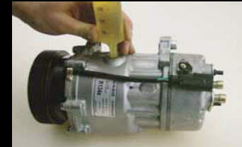
5. Adjust oil quantity according to manufacturer's advice
